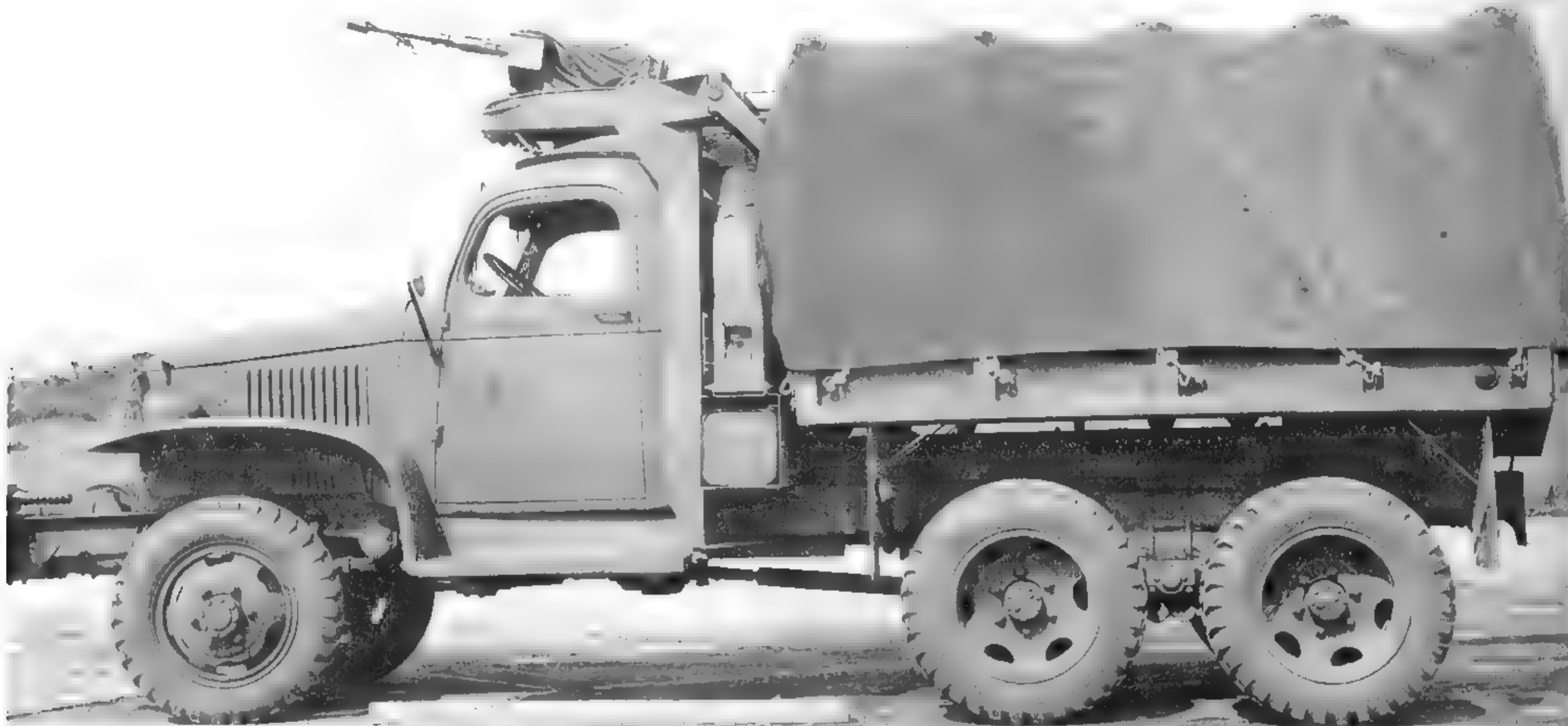
Some of the short-wheelbase CCKWs were built with winches, and some had M32 ring mounts installed on them. This truck is one of a fairly small percentage that were equipped with both. (National Archives and Records Administration photo collection)
